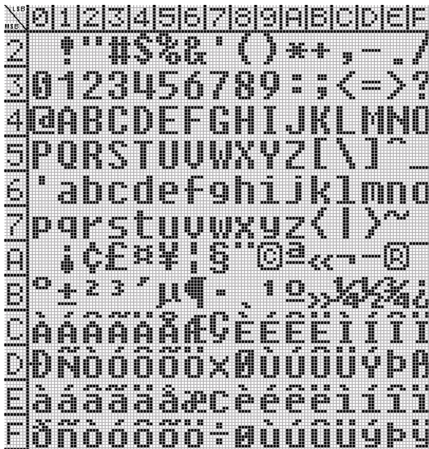
Code Map, Serial Controller ISO/IEC 8859-1 Compliant 10 Row font
